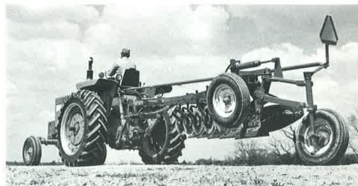
Travel safely in road gear. Tail wheel carries part of the plow's weight. This increases stability on the highway as well as when making field turns.
