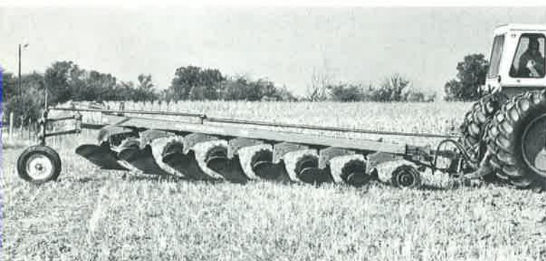
You get fast penetration regardless of ground conditions . . . just lower the front of the plow to pitch bottoms down so points bite in fast.
