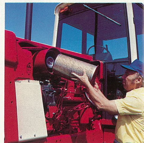
Dry-type, dual stage air cleaner has an automatic dirt unloader, plus cleanable element and final built-in secondary element.
