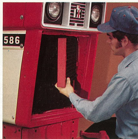
Swing-out air conditioner condenser and oil cooler at front of radiator are fully accessible.
