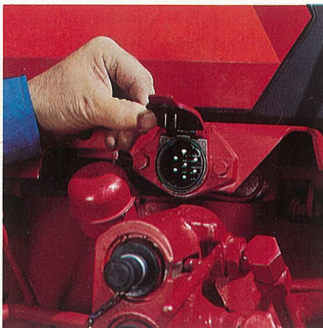
Quick disconnects outside of control center for electrical wiring.
