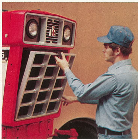
Single latch grille is easily removed.
