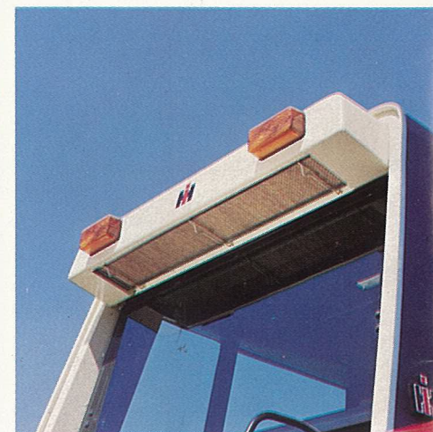
Self-purging, back-flush filter system outside of control center. Easy filter changing.
