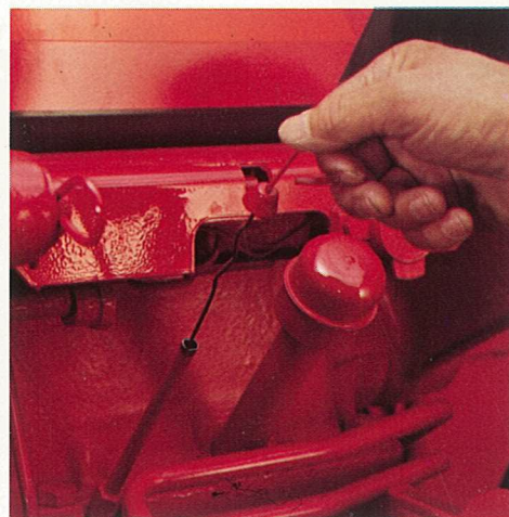
Transmission, differential and hydraulic oil reservoir filler tube located outside of control center and easily accessible.
