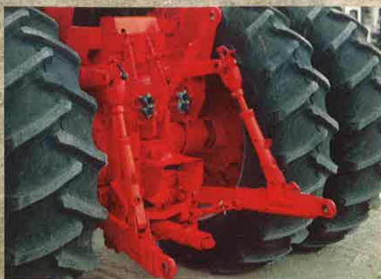
3-point hitch attachment includes swinging drawbar. Tractor at right is equipped with new Quick Coupler for 3-point hitch . . . for implement hook-up from the tractor seat. Both hitch and coupler are Category III convertible to II.
