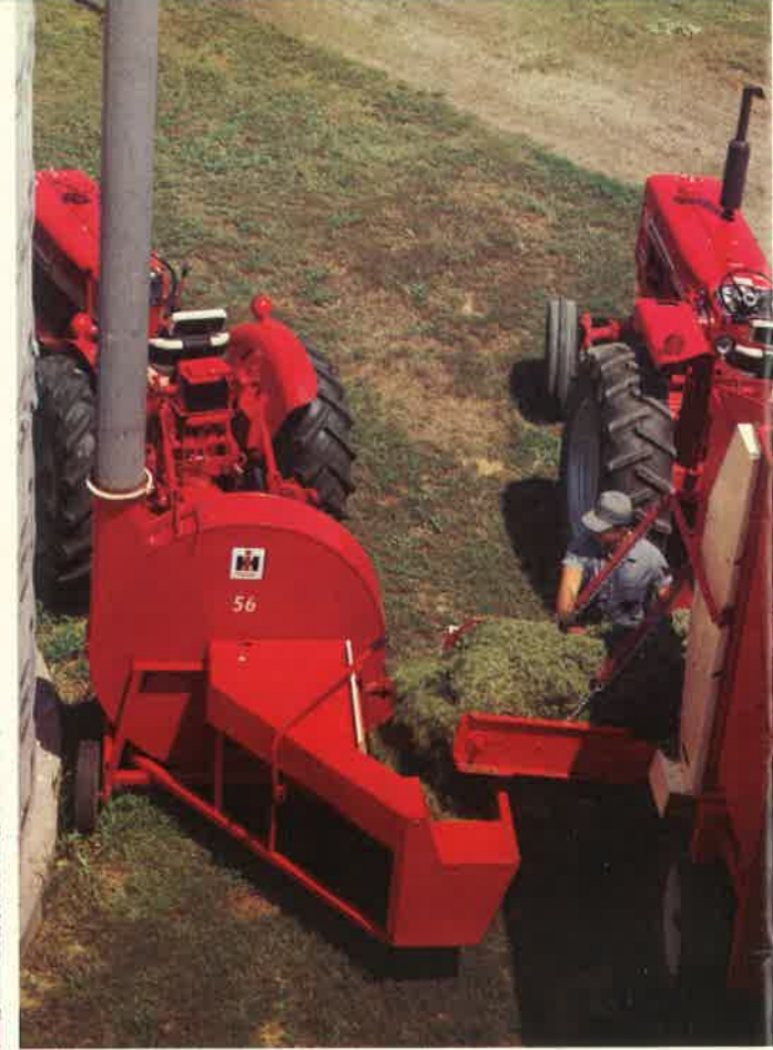
56 blows 100 tons corn silage, or 70 tons haylage an hour.
