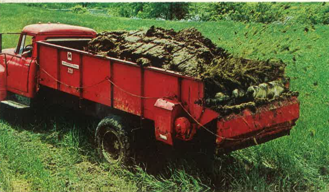
Endgate (130, 155 & 175)—Low-cost, snug-fitting mechanical endgate helps hold soupy manures.
