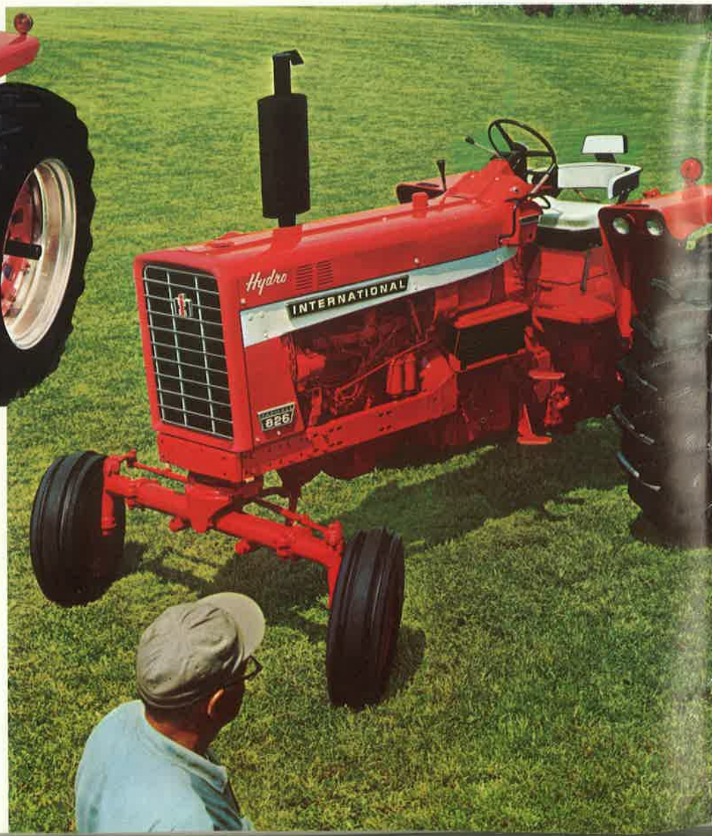
INTERNATIONAL 826 HYDROSTATIC. 84 H.P. pto (Mfr. est. max.). Choice of 358 cu. in. diesel or 301 cu. in. gas engines.
