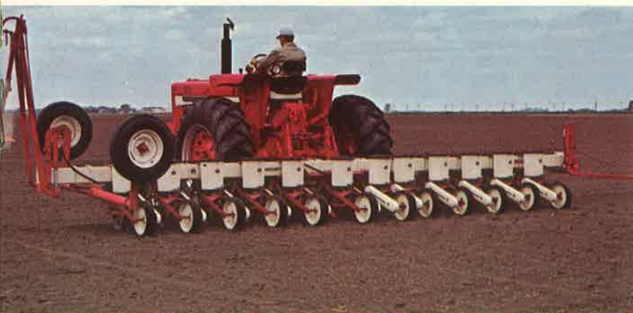
Twelve 295 Planter Units mounted on a 326 Planter Carrier plant beets in 20-inch rows in Minnesota.
