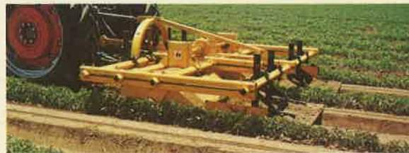
712 FURROW MULCHERS incorporate post emergence herbicide in-between the beds. For wide spaced crops such as tomatoes, the "712" is the ideal machine for breaking up clods, final forming of uniform beds and cultivating the furrows.
