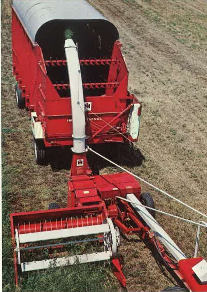
350 chops up to 40 tons of corn an hour; chops as fine as 3/16-in.
