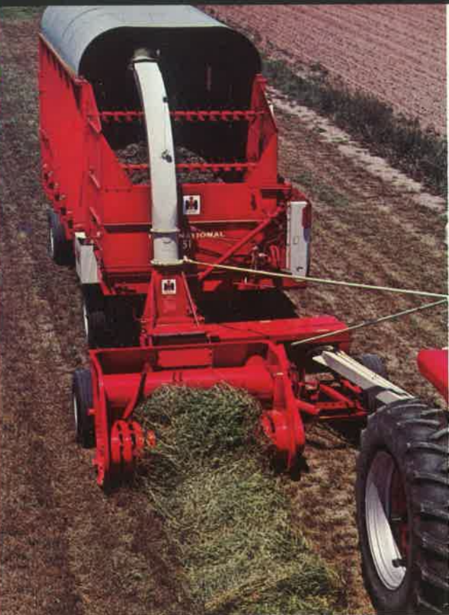
350 chops up to 80 tons of corn an hour; chops as fine as 1/8-in.
