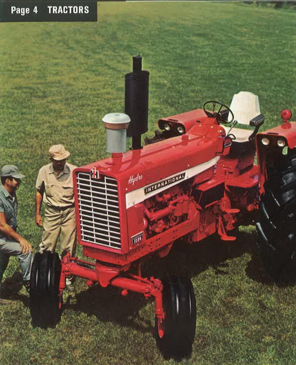
INTERNATIONAL 1026 HYDROSTATIC. 112 H.P. pto (Mfr. est. max.). 407 cu. in. turbo diesel engine.
