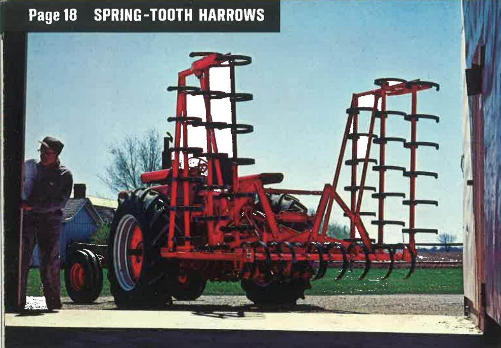
340 MOUNTED SPRING-TOOTH HARROW. The tough, dependable 340 is built to withstand the stress of high-speed, maximum depth work. Being fully-mounted, it permits you to take full advantage of draft control for keep-going farming. Hinged sections provide greatest flexibility for working rough or uneven fields. Hydraulic folding models from 16 to 21-foot sizes . . . non-folding models from 7 to 14-foot sizes. 4½ or 6-inch tooth spacing.
