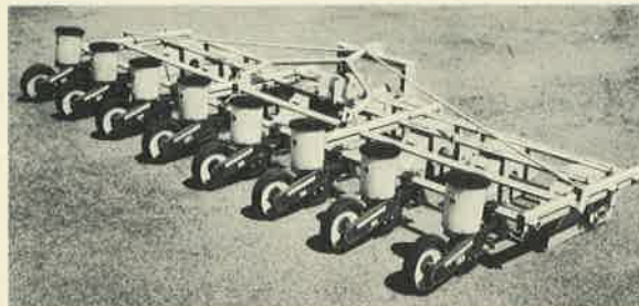
704 MOUNTED INCORPORATOR , designed for both bedded and flatland farming, will mulch and incorporate herbicide. Available in 2, 4, 6 or 8 row models with 3 or 4 tool bars . . . planters and ground-working tools can be added. The "703", similar in design, is primarily used in sugar beets and beans. Available in 4 or 6 row models for 22 to 24 inch row spacing.
